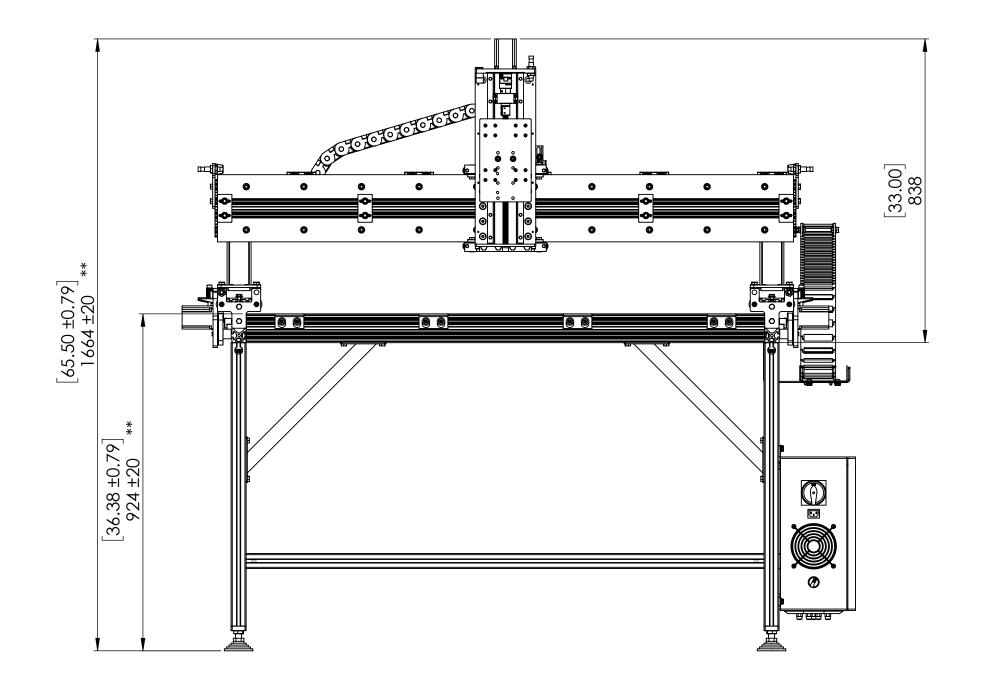
12" Travel Z-Axis will add 100mm (3.94") to top of machine \*\*Adjustment of leveling feet in leg kit will impact actual height dimension
