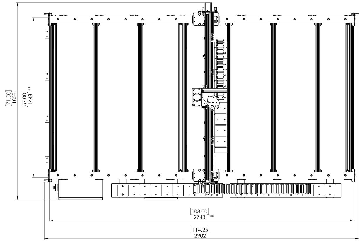
\*\*Dimension to outside edges of extrusion, use this measurement if building your own leg assembly
