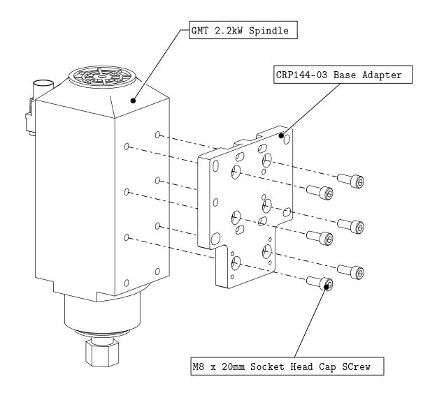
• Attach the spindle to the base adapter as indicated.
