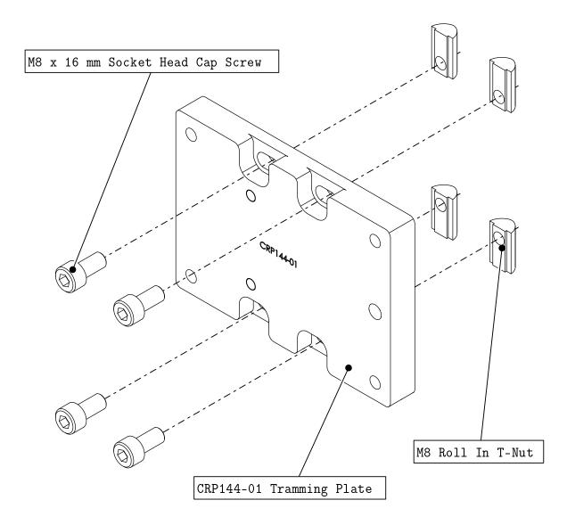
• Thread the socket head cap screws into the t-nuts through the tramming as indicated
