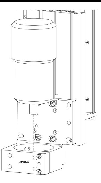
• Slide your router or round spindle into the router mount as indicated.
