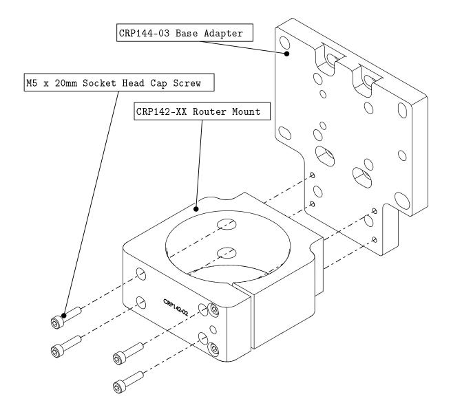
• Attach the router mount to the base adapter as indicated
