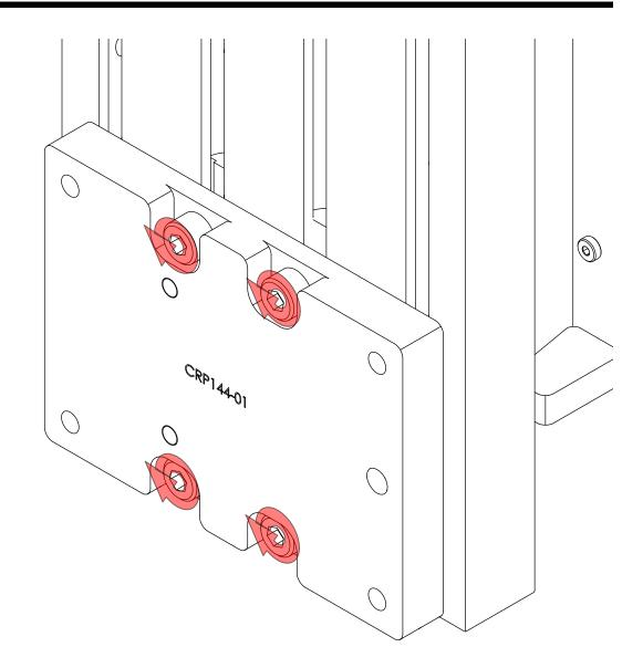
• Tighten the highlighted fasteners.
