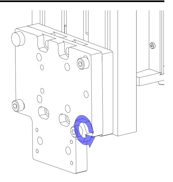
• After completing test cuts, you may slightly loosen all four of the mounting fasteners, and rotate the eccentric bearing to adjust your tram.
