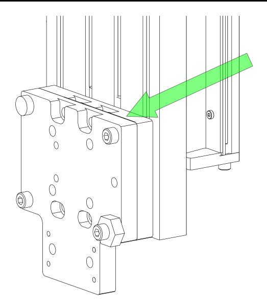
• In most installation, tram does not need to be adjusted around the axis parallel to the gantry of the machine. However, if adjustment is required in this direction, a small shim can be placed between the tramming plate and the base adapter, at the top or bottom as needed.
