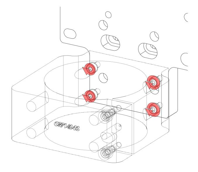
• Tighten the highlighted fasteners.
