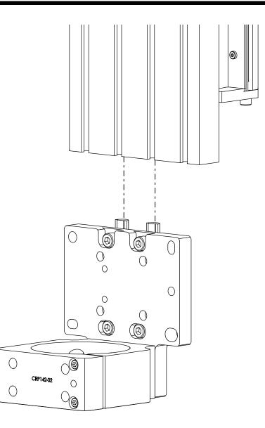
• Slide the router mount assembly into the t-slots of the z axis as indicated.
