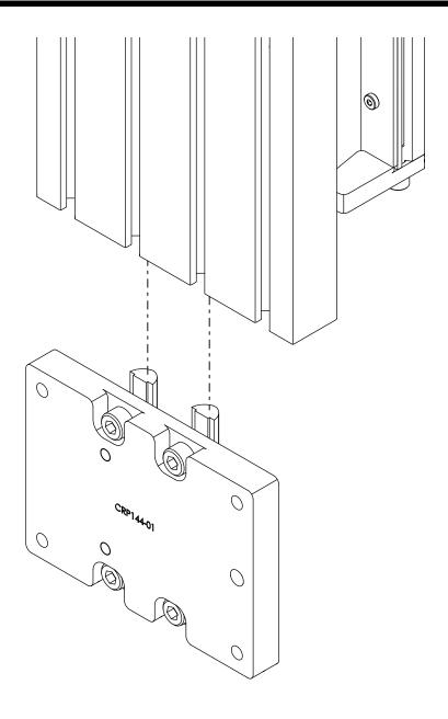
• Slide the tramming plate into the t-slots of the z axis as indicated.
