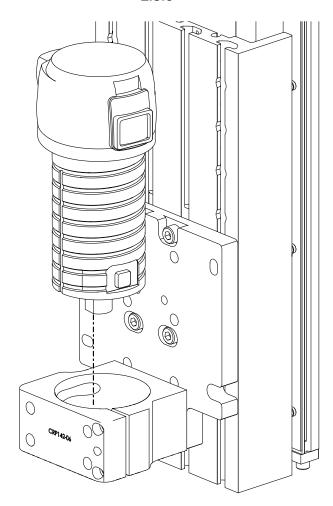
• Slide your router or round spindle into the router mount as indicated.
