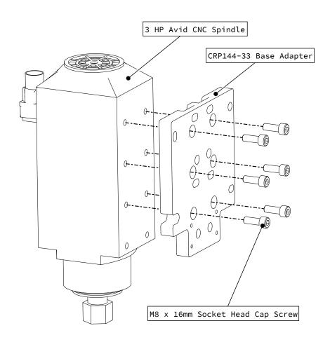
• Attach the spindle to the base adapter as indicated.
