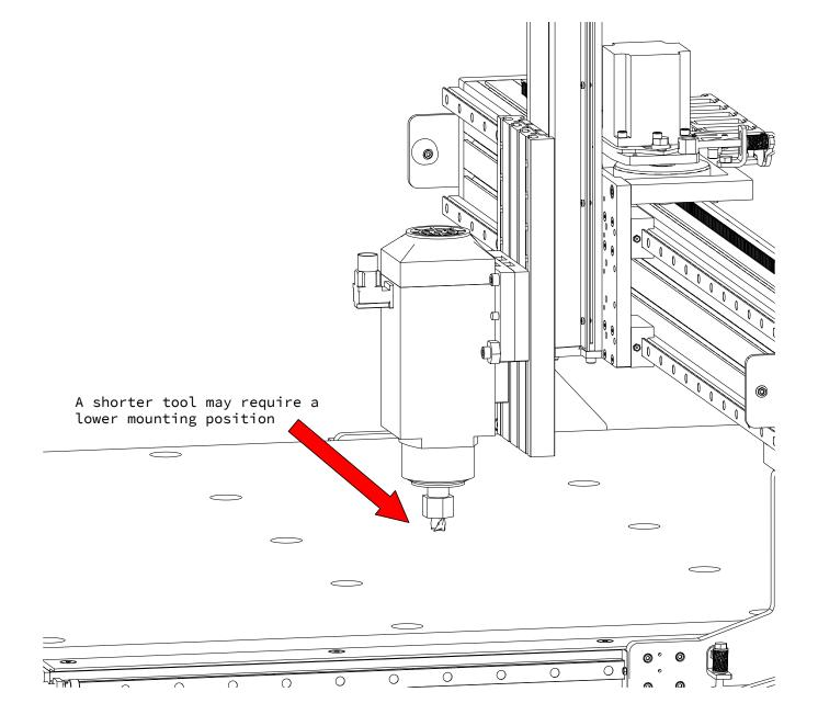
If shorter tools are commonly used, it may be necessary to position the router or spindle in a lower position. Whatever mounting position you choose, it is recommended to mount the base adapter/tramming plate in the highest position possible while still allowing the vertical range required.
