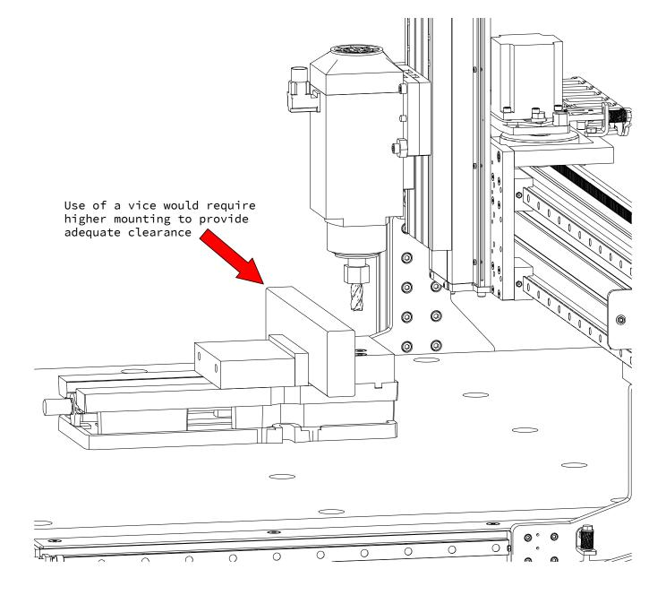
Many situations will require a different mounting location than the one specified in these instructions. For example if a vise is used to hold work pieces, a higher mounting position may be required.
