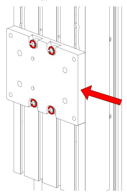
• While pushing on the tramming plate in the indicated direction, fully tighten the tramming plate fasteners.
