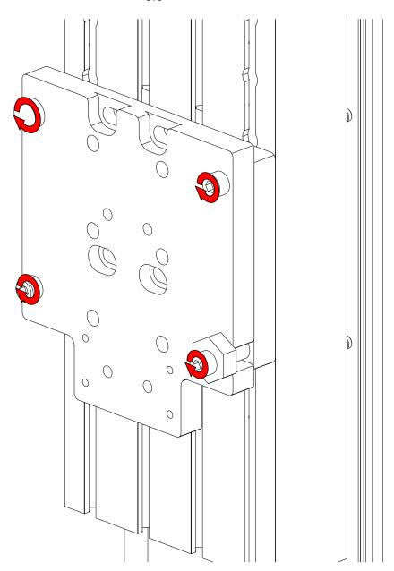
• Tighten the highlighted fasteners.
