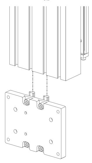
• Slide the tramming plate into the t-slots of the Z-Axis as indicated.
