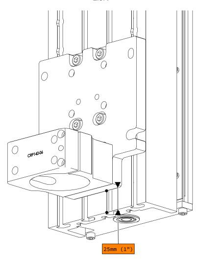
• Position the base adapter 25mm (1") from the bottom of the Z-Axis moving plate as indicated.
