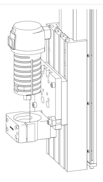
• Slide your router or round spindle into the router mount as indicated.
