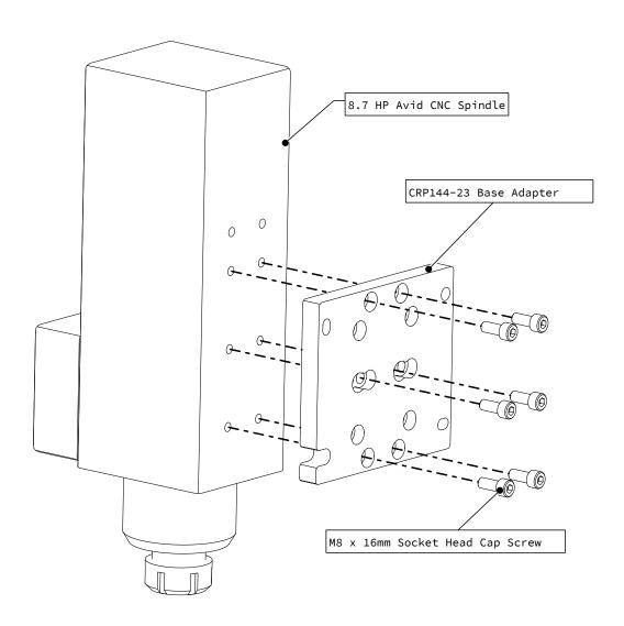
• Attach the spindle to the base adapter as indicated.
