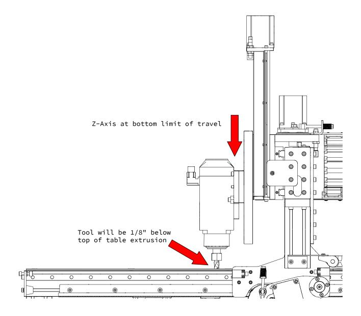
The examples above applies for a PRO CNC machine configured with an 8" Z-Axis and 8" Gantry Height, using a tool with a length of 1.5". If you are using a different machine configuration or tool length, you will need to adjust your router or spindle mount location accordingly.
