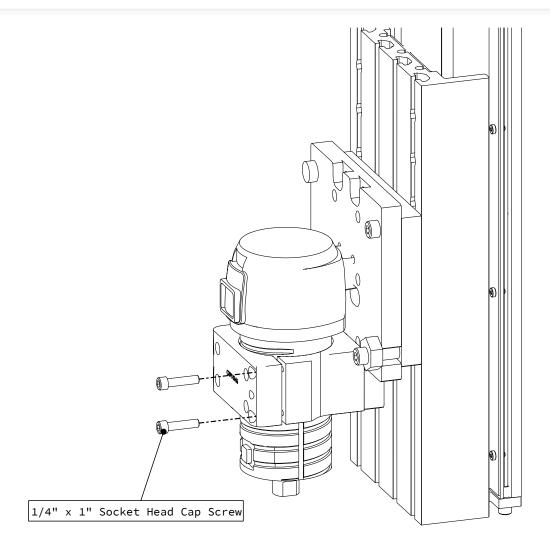
• Install the clamping fasteners as indicated.
