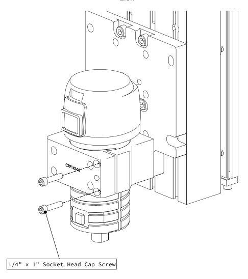
• Install the clamping fasteners as indicated.
