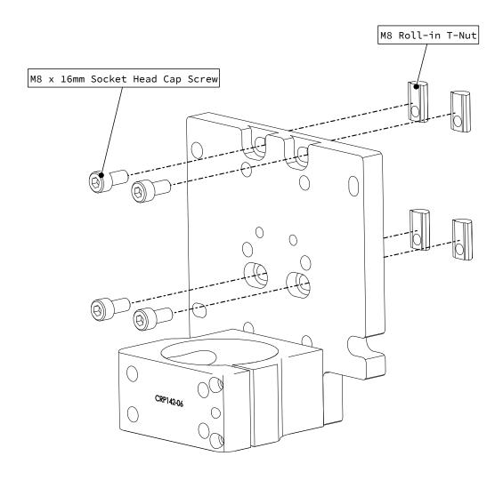
• Partially thread t-nuts onto the socket head cap screws as indicated.
