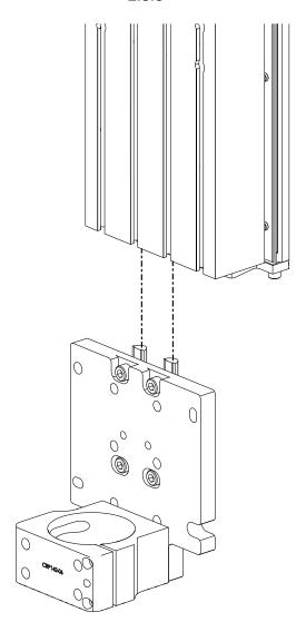
• Slide the router mount assembly into the t-slots of the Z-Axis as indicated.
